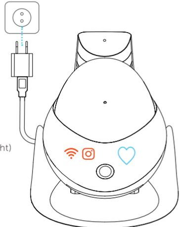
Place REDDY on the charging dock. If indicators are not lit, reboot the robot's settings by pressing Reset button for 5 sec, then turn the robot on by pressing Reset button for 2 sec
